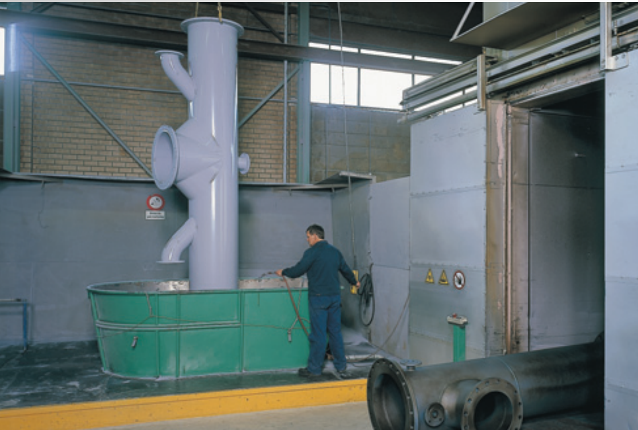
Oven and dipcoat installation
